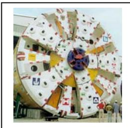
**The 4<sup>th</sup> River Elbe Tunnel** was a milestone in Slurry-TBM tunneling due to the large TBM diameter of 14.2 m, low cover of as small as 7 m and high groundwater pressure of up to 4.5 bar. The southern section of the 2,561 m long tunnel was excavated in glacial deposits consisting of sand, marl and boulders, while more cohesive ground such as marl and clay with sand lenses and boulders was present on the northern tunnel section.
