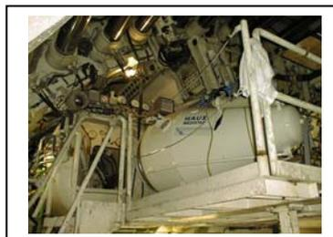
The 4<sup>th</sup> River Elbe tunnel was the first project where a rescue could be completed by connecting a NATO lock on the TBM to enable transport compressed air pressure to a shuttle surface. Fortunately it was not
