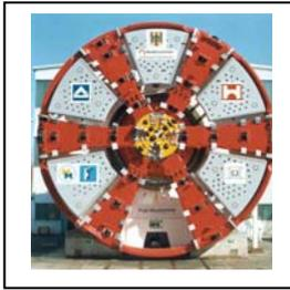
The 1.640 m long twin tube **Wesertunnel** crosses the river Weser north of Bremen, Germany. A Slurry-TBM ( $\varnothing$  11.71 m) was used to excavate the tunnel in glacial deposits. The glacial soil consists of poorly graded and partly very loose cohesion, less sand with hard granite boulders, and very soft to soft clay and peat in shallow areas. Below the river, plastic clays were found to have mainly stiff to hard consistency reaching shear strength values of weak rock.
