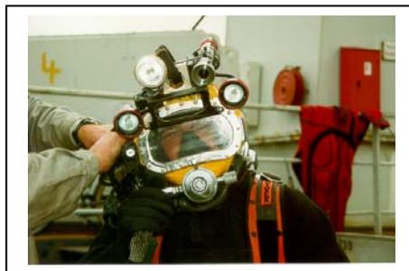
Diving helmets normally used for offshore diving were specially modified to allow them to be used for diving in bentonite. To make it easier for the divers to breathe in the bentonite, which is a clay suspension, and to reduce breathing resistance, the helmets were fitted with a water flushing system for the air regulator. The constant supply of fresh water also prevents the breathing membranes from sticking together.
