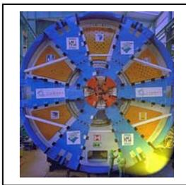
The 6.6 km long **Westerschelde Tunnel** is the first tunnel project where saturation diving technique was used for excavation chamber interventions. The twin tube tunnel was excavated by two Slurry-TBMs ( $\varnothing$  11.33 m). Ground conditions consist of medium to fine quaternary sands within shallow sections and a massive formation of tertiary stiff clay on a length of approx. 2 km. Dense tertiary sands are found below the clay within the deepest tunnel section.
