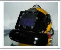
For the welding operation we use the new special designed compressed air helmet with triple air supply, two regulators and one free flow, communication, camera and an integrated welding shield with sensors.
