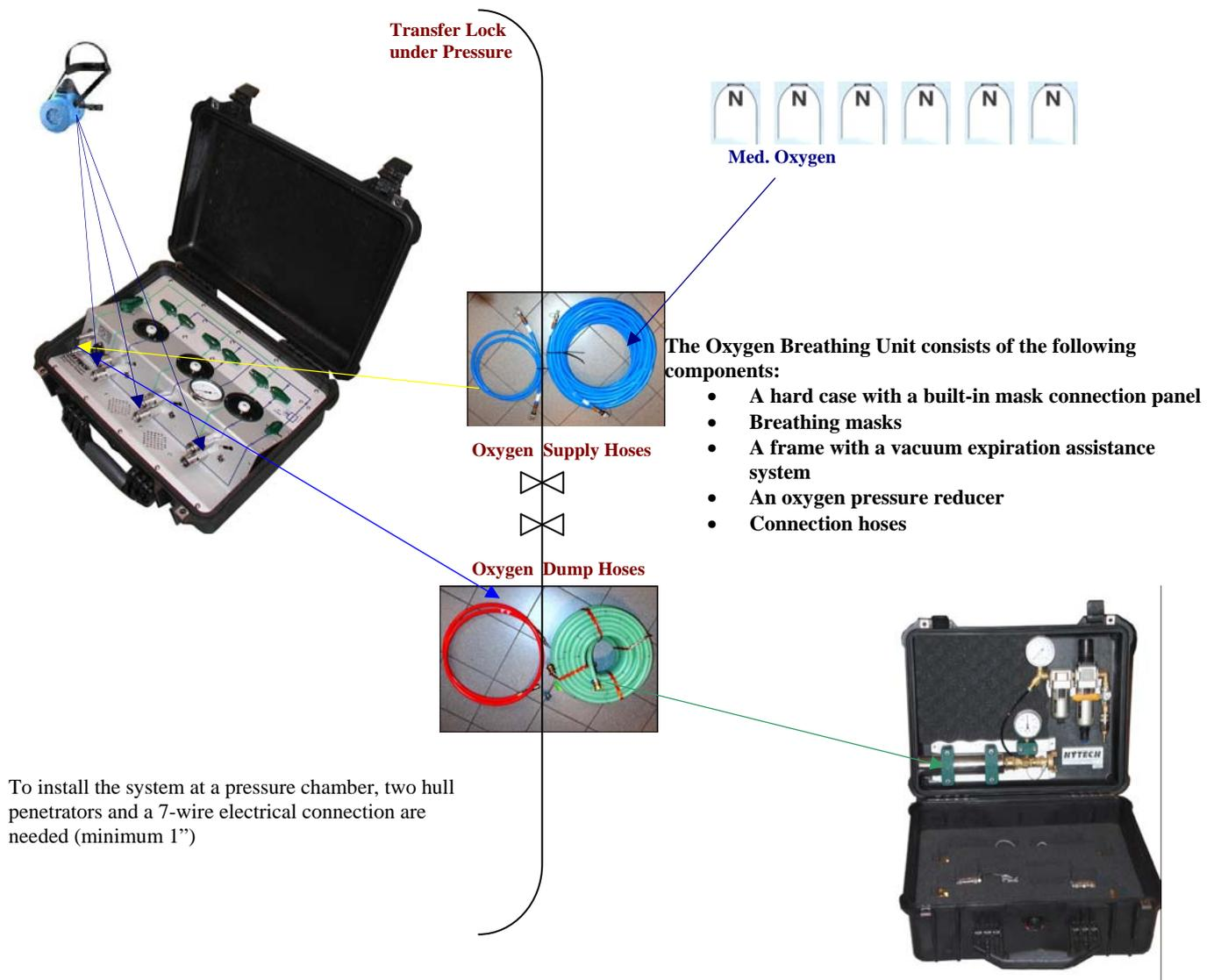
The Frame can be placed at a safe location to dump the exhaled oxygen. The frame is connected to the pressure chamber with a large diameter exhaust hose.
