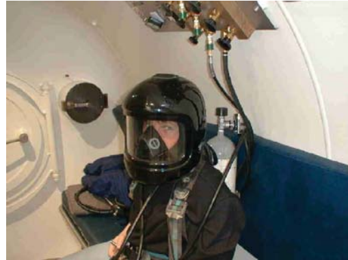
Figure 10. Special diving helmet (hyperbaric helmet) for application in hyperbaric conditions at 6.9 bars.
